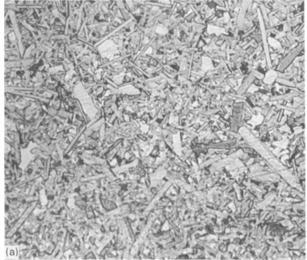
Figure 6 Polished surface of 10 wt% alumina sample, sintered at 2050°C for 30 min under CO pressure.
